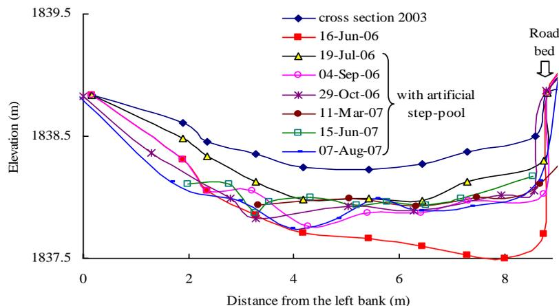
**Fig. 6** Fluvial processes at a cross section in the experimental reach of the Diaoga River with an artificial step-pool system, which was constructed on June 16–18, 2006
